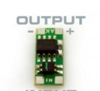
This new and unbelievable small constant current power supply for your LEDs works with the above mentioned output current. The forward voltage is secundary. This garanties a homogeneous brightness through the whole forward voltage range and a maximum lifetime to the connected LEDs.
