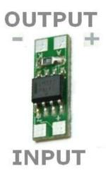
This new and unbelievable small constant current power supply for your LEDs works with the above mentioned output current. The forward voltage is secundary. This garanties a homogeneous brightness through the whole forward voltage range and a maximum lifetime to the connected LEDs.
