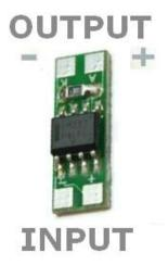
This new and unbelievable small constant current power supply for your LEDs works with the above mentioned output current. The forward voltage is secundary. This garanties a homogeneous brightness through the whole forward voltage range and a maximum lifetime to the connected LEDs.
