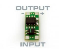
This new and unbelievable small constant current power supply for your LEDs works with the above mentioned output current. The forward voltage is secundary. This garanties a homogeneous brightness through the whole forward voltage range and a maximum lifetime to the connected LEDs.
