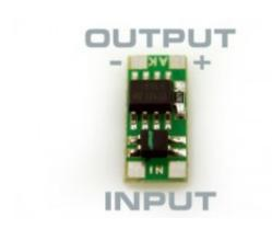
This new and unbelievable small constant current power supply for your LEDs works with the above mentioned output current. The forward voltage is secundary. This garanties a homogeneous brightness through the whole forward voltage range and a maximum lifetime to the connected LEDs.
