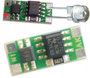
mA typ.: 100 mA V typ.: 38 V with the above mentioned output current. The forward voltage is secundary. This garanties a homogeneous brightness through the whole forward voltage range and a maximum lifetime to the connected LEDs.
